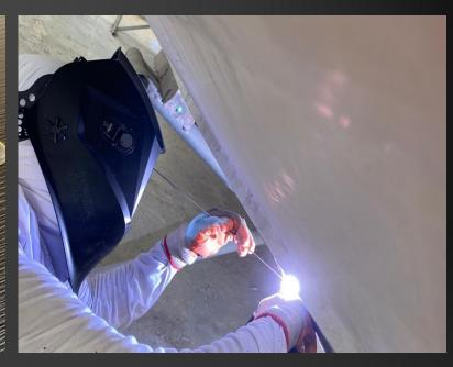
WE HAVE A DEDICATED STEEL FABRICATION AREA WITH MASTER TIG WELDERS AND FABRICATORS FOR MARINE 5083 ALUMINIUM AND 316 STAINLESS APPLICATIONS.
